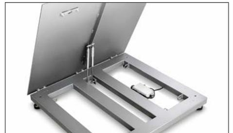
Cavities and concealed edges are avoided by using hermetically welded section tubes. When combined with the clever frame structure, which reduces potential contamination areas, the result is a floor scale design which is of special benefit when used in areas where hygiene is particularly important.
