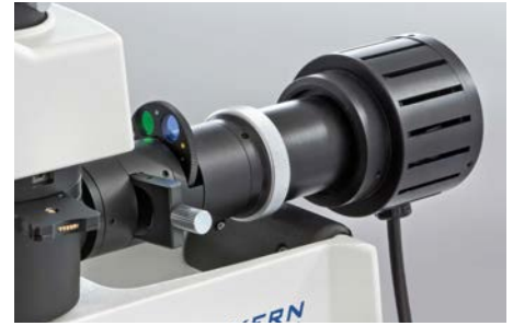
Illumination unit with filter disc
